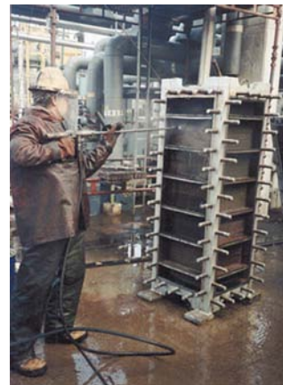
Figure 2. An operator effectively cleans the Compabloc.
