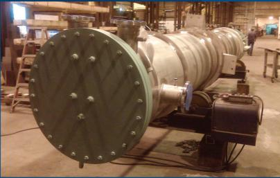
For over 40 years, Enerquip has been providing both standard and custom shell & tube heat exchangers to our industrial customers. Our reputation for high quality and fast lead-times have earned the trust of many top companies in the chemical, pulp/paper, waste water, military, power, renewable energy and refining markets.
