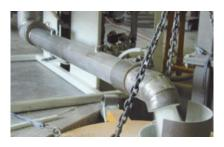
Stinger media can be used to line piping or bin bottoms to solve bridging and flow issues. The Stinger gently lifts the powders off of the wall of the pipes or vessels via air or gas and allows powders to take on the flow characteristics usually seen in liquids. The result is fast conveying on your powders without the moving mechanical parts which
